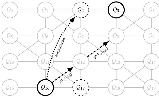
**Figure 6: Teleportation vs. swapping for  $CNOT(Q_3, Q_{16})$**
