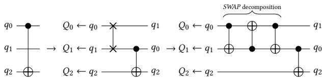
Figure 3: Mapping and decomposition using SWAP gates
