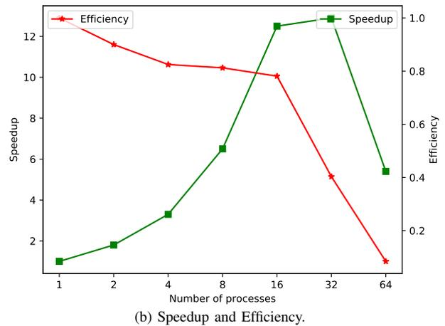
Fig. 8: Absolute execution time, speedup and efficiency of the whole simulation.
