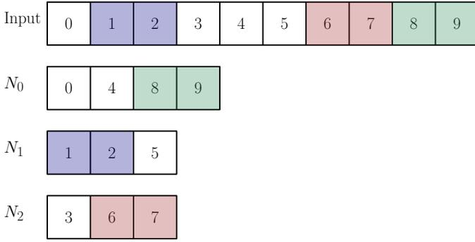
Fig. 4: Partition of the input data to three processes. Colored fields mark identical values.
