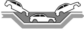
Fig. 1: A simplified Electrodeposition tank used in automotive industry to apply coatings.
