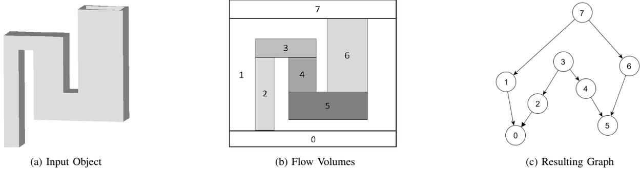
Fig. 2: Geometric decomposition of a simple object.
