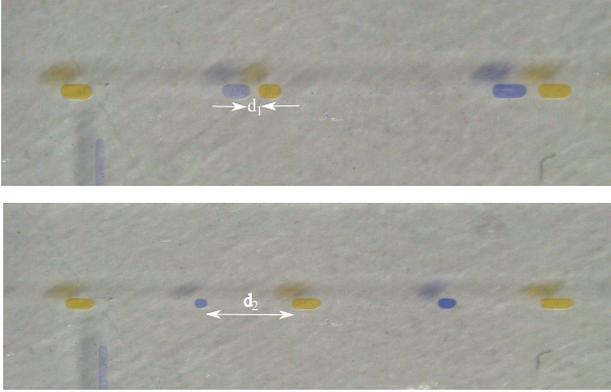
Fig. 2. Practical realization of header-payload droplet generation using DbD encoding mechanism. The distance between the droplets was dynamically changed from  $d_1$  to  $d_2$  using the DoD system.
