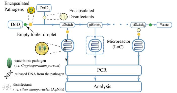
Fig. 3. Fast and flexible pathogen screening using microfluidic networks
