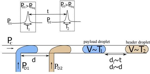
Fig. 1. Illustration of cascaded DoD system for generating payload-header droplets
