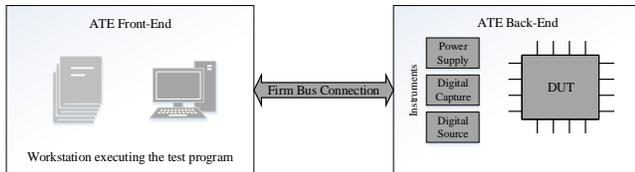
Fig. 2: Automatic Test Equipment (ATE).
