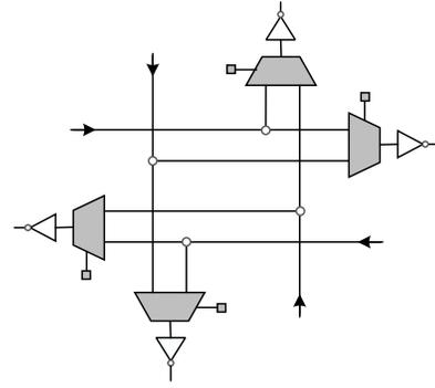
Fig. 6: Scenario- $\{EN, NW, WS, SE\}$  switch-box architecture.
