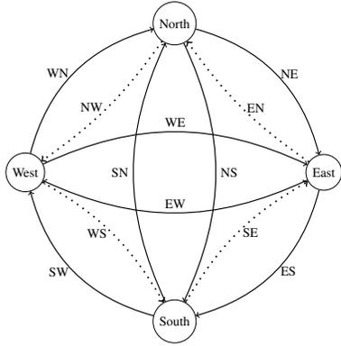
Fig. 5: Possible turns realized by a switch-box.
