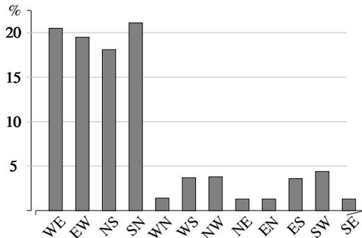
Fig. 4: Utilization of switch-box turns.
