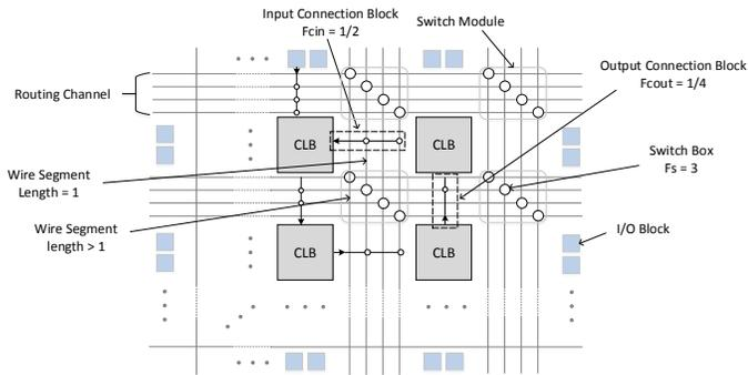
Fig. 2: Architecture of an island-style FPGA.
