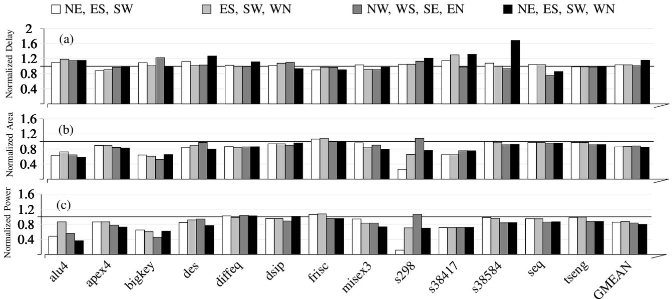
Fig. 7: Obtained results normalized to the baseline; (a) Normalized Delay, (b) Normalized Area, and (c) Normalized Power.
