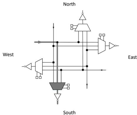
Fig. 3: Unidirectional mux-based switch-box.
