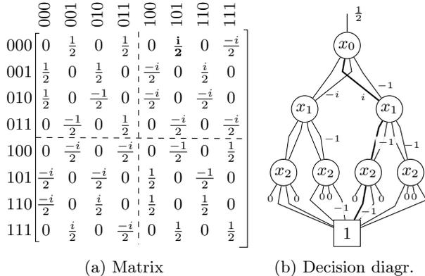
Figure 1: Matrix and dec. diag. of a 3-qubit computation
