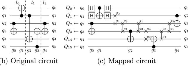
Figure 2: Mapping of a circuit to the *IBM QX3* architecture
