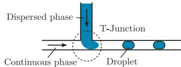
**Fig. 3.** Generation of droplets using a T-junction.
