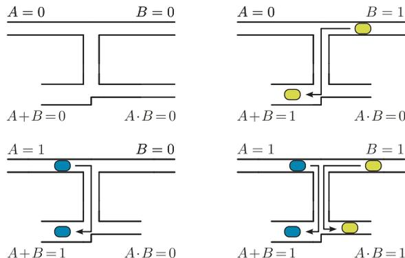
**Fig. 4.** Working principle of a microfluidic AND/OR gate [6].
