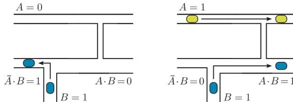
**Fig. 5.** Working principle of a microfluidic AND/NOT gate [6].
