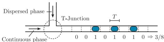
**Fig. 6.** Droplet stream representing the number  $3/8$ .
