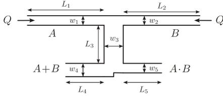
**Fig. 7.** Layout of AND/OR gate.
