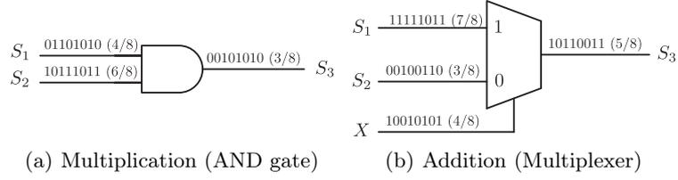
**Fig. 2.** Logic circuits for performing arithmetic operations in SC [7].
